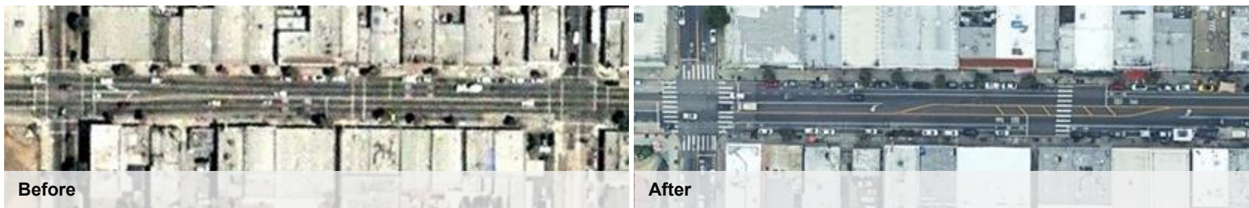
Figure 18: York Boulevard Before and After Lane Reconfiguration
