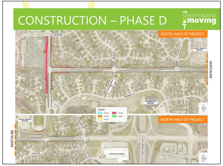
During Phase D, shown in Pink, traffic on Pacific Street will be shifted head-to-head on the newly constructed pavement on the north side of the road. The south half of Pacific Street will then be constructed.
