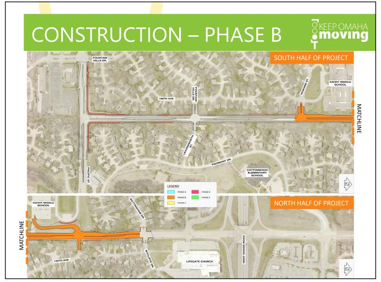
In Phase B, shown in Orange, 156<sup>th</sup> Street from Howard Street to Wycliffe Drive will be closed to traffic and reconstructed. The start of the phase will not be allowed to start until Millard Public Schools goes on summer break. This phase has several subphases to ensure at least 2-lanes of 156<sup>th</sup> Street can be completed and reopened prior to Kiewit Middle School starting in the August. The Contractor has until the Fall of 2023 to complete all of Phase B.
