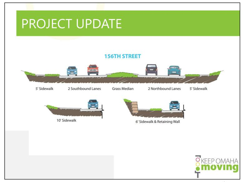
This graphic shows what the typical cross section of the proposed 4-lane divided roadway would look like on 156<sup>th</sup> Street. It will include 2-lanes in each direction separated by a raised median and a 5 foot sidewalk on both sides of 156<sup>th</sup> Street.
