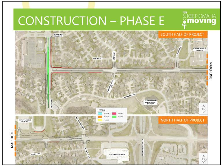
The final phase, Phase E shown in Green, is construction of center lanes and medians in the central portion of Pacific Street. Traffic will be open in both directions for Pacific Street but shifted to outside lanes. The Contractor has until Late Spring of 2024 to complete this Phase.
