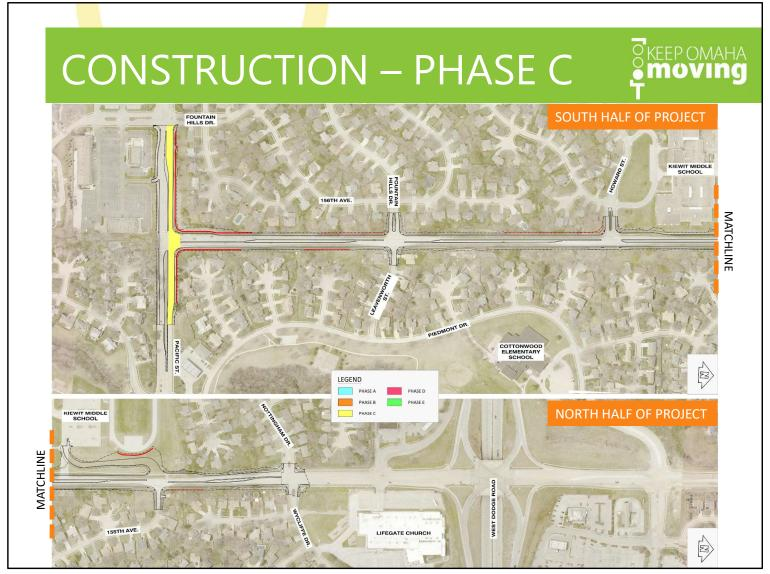
In Phase C, shown in Yellow, Pacific Street traffic will be shifted head-to-head on the south side of the roadway. The north half of Pacific Street improvements will then be constructed in this phase.
